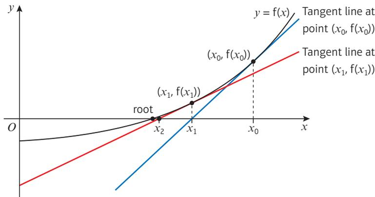
If the starting value is not chosen carefully, the Newton–Raphson method can converge on a root very slowly, or can fail completely. If the initial value,  $x_0$ , is near a turning point or the derivative at this point,  $f'(x_0)$ , is close to zero, then the tangent at  $(x_0, f(x_0))$  will intercept the  $x$ -axis a long way from  $x_0$ .
