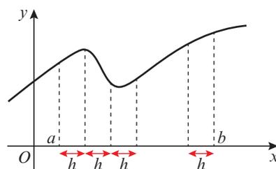
Next you calculate the value of  $y$  for each value of  $x$  that forms a boundary of one of the strips. So you find  $y$  for  $x = a, x = a + h, x = a + 2h, x = a + 3h$  and so on up to  $x = b$ .
