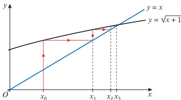
Read up from  $x_0$  on the vertical axis to the curve  $y = \sqrt{x + 1}$  to find  $x_1$ . You can read across to the line  $y = x$  to 'map' this value back onto the  $x$ -axis. Repeating the process shows the values of  $x_n$  converging to the root of the equation  $y = \sqrt{x + 1}$ , which is also the root of  $f(x)$ .
