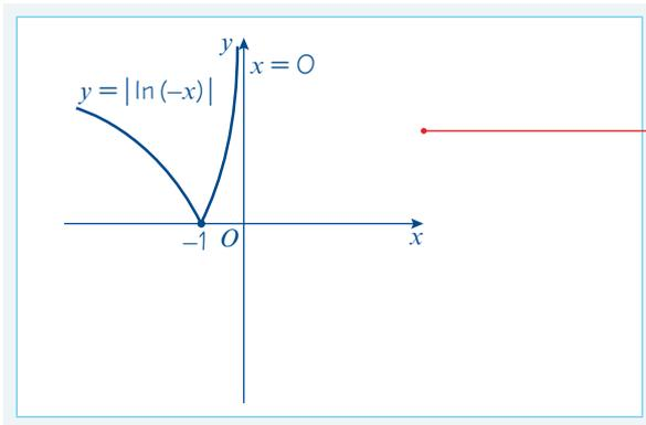
To sketch the graph of  $y = |f(-x)|$  reflect any negative  $y$ -values of  $y = f(-x)$  in the  $x$ -axis.
