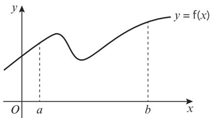
To approximate the area given by  $\int_a^b y \, dx$ , you can divide the area up into  $n$  equal strips. Each strip will be of width  $h$ , where  $h = \frac{b - a}{n}$
