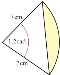
$$\begin{aligned} \text{Area of segment} &= \frac{1}{2} \times 7^2(1.2 - \sin 1.2) \\ &= \frac{1}{2} \times 49 \times 0.26796\dots \\ &= 6.57 \text{ cm}^2 \text{ (3 s.f.)} \end{aligned}$$
