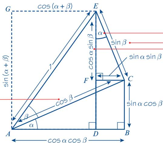
$$\angle ACF = \alpha \Rightarrow \angle FCE = 90^\circ - \alpha. \text{ So } \angle FEC = \alpha.$$
