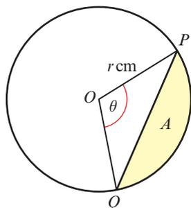
Using  $\frac{1}{2}r^2\theta$  for the area of the sector and  $\frac{1}{2}ab \sin \theta$  for the area of a triangle:
