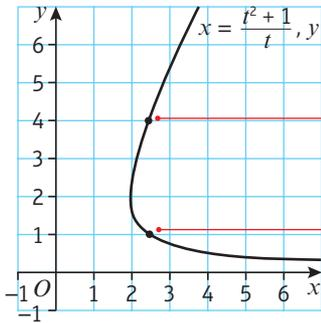
These are the parametric equations of the curve. The domain of the parameter tells you the values of  $t$  you would need to substitute to find the coordinates of the points on the curve.
