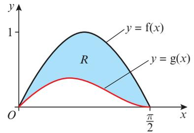
$$\begin{aligned} \text{Area} &= \int_a^b (f(x) - g(x)) dx \\ &= \int_0^{\frac{\pi}{2}} (\sin 2x - \sin x \cos^2 x) dx \\ &= \left[ -\frac{1}{2} \cos 2x + \frac{1}{3} \cos^3 x \right]_0^{\frac{\pi}{2}} \\ &= \left( -\frac{1}{2}(-1) + \frac{1}{3}(0) \right) - \left( -\frac{1}{2} + \frac{1}{3} \right) \\ &= \frac{2}{3} \end{aligned}$$
